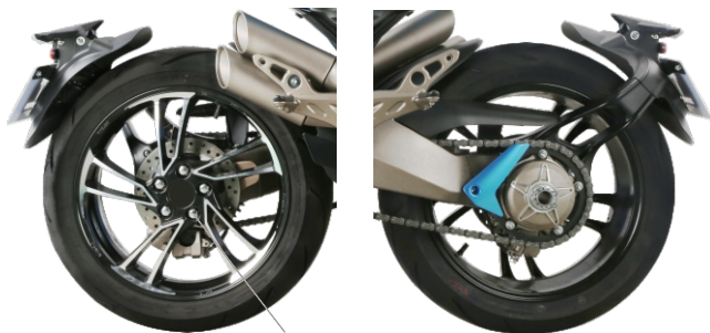
M12×1.5 nuts Rear wheel nut tightening torque: 110N.m
